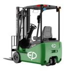
TCL is a compact 80V lithium-ion 3 wheels forklift designed for applications in tight indoor spaces, offering small turning radius and a low overall height that enables work in narrow aisles, low-clearance areas, mezzanines, and cargo lifts. Its dual-drive PMS Motor ensures smooth, agile handling, while automatic stop on ramp and speed reduction on turns support safe operation. TCL is the ideal forklift for light to medium-duty applications where maneuverability are the main priorities.
