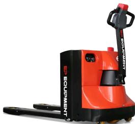
The EPT25-WA is ideal for high-intensity pallet transport in distribution centers, warehouses, and loading docks. Its anti-rollback brake, emergency disconnect, and automatic speed reduction features make it a safe choice for operators. Optional cold storage configuration expands its versatility to frozen food and pharmaceutical supply chains.
